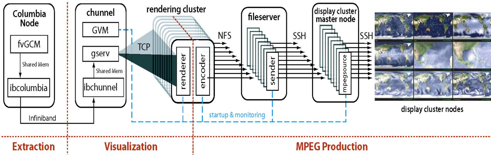
*The NASA ARC Concurrent Visualization System. Rounded rectangles indicate systems, and rectangles indicate processes. The whole system (from left to right panels) consists of a computing node ("Columbia node"), a 16-CPU middle-layer system ("Chunnel"), 50 dual-CPU rendering cluster, and the hyperwall-1. These systems are used for data extraction, data handling, data visualization and MPEG image production, and visualization display.*
